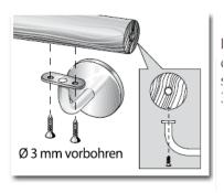
Screw the handrail support with the support in the **groove** of the handrail. (Countersunk screw 3.5x25 mm)
