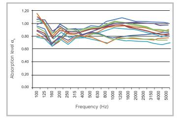
dukta<sup>®</sup> corrugated acoustic walls and ceilings reach, across all frequencies, as high sound absorption values as other products in specific frequency ranges.
